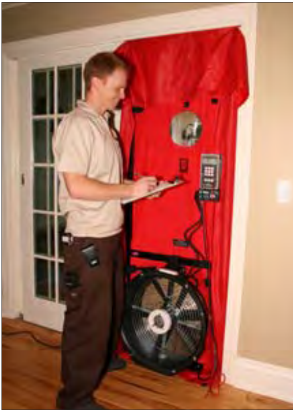
EA51 Blower Door Test Set-Up
